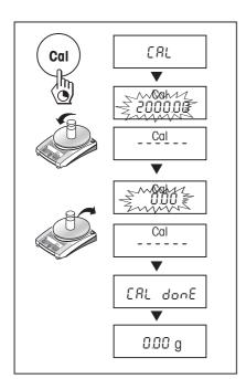
To obtain accurate results, the balance must be left switched on for 60 minutes to reach operating temperature before starting the adjustment procedure.
