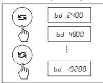
The baud rate (data transfer rate) determines the speed of transmission via the serial interface. The unit is the baud (bd) = 1 bit/second.
